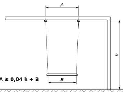
**A** distance between the suspension points along the crossbeam.
